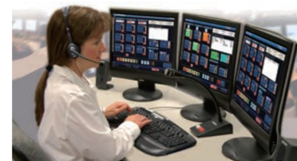
Desktop Wireless Console System (Zetron) A radio control operation device (desktop terminal) that allows remote control and communication of wireless devices located at a distance from an office or workplace, just like a telephone.
