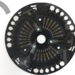
Testing cartridge φ120mm t1.2mm
