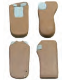
Clay mockups used to research ease of handling
