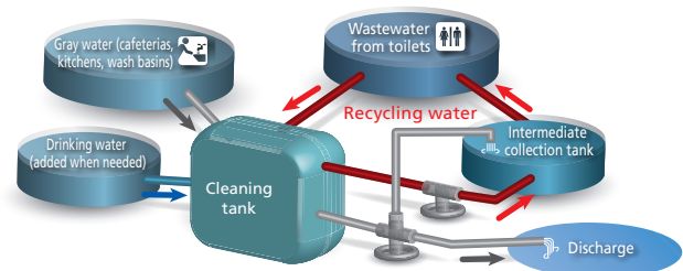
Using recycled water at the Head Office & Yokohama Business Center to reduce water usage
