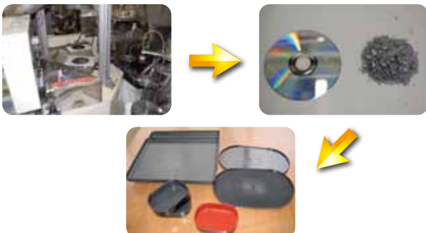
Disks that fail the quality inspection are sent to subcontractors after destruction to be recycled as materials for lacquered containers
