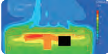
Heat analysis technology is used to optimize component layout which allows for a smaller radiator
