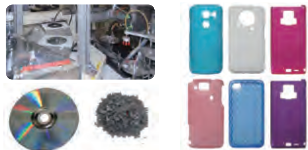
Disks that fail the quality inspection are pulverized and recycled as cases for smart phones
