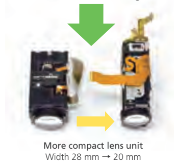
Strength analysis allows lens units to be reduced in size without sacrificing durability
