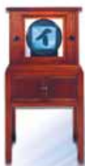
1939: The first commercial television receiver in Japan. The Japanese katakana character “イ” was the first ever image on the CRT.
