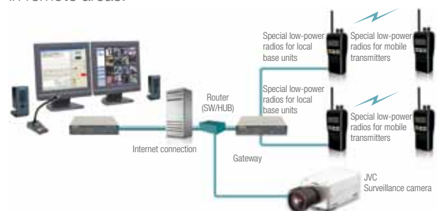
"VoIP radio dispatch system" developed by Zetron
