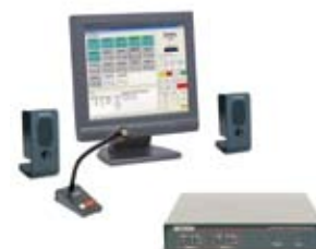
[8] VoIP radio dispatch system
