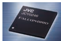
⑥ JVC LSI enables high-speed image processing in HD camcorders
