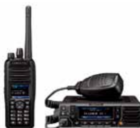
2. NEXEDGE NX-5000 series of multi-mode digital radio systems that are compliant with the P25 standard
