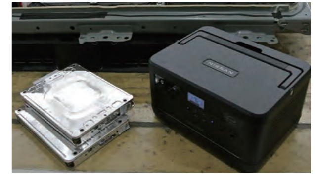
Recycled Nissan LEAF battery cells that will be used in the product (left) and the product image under development (right)
